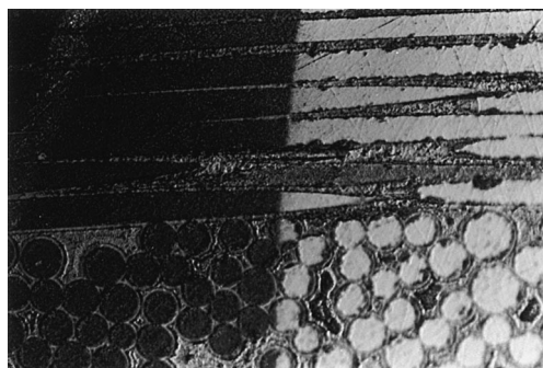
Fig. 2. Optical microscope image of helium implanted SiC/SiC composite after annealed at 1673 K.
